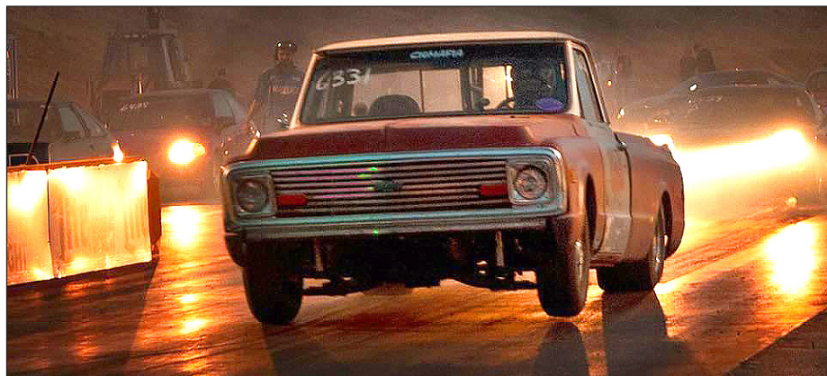
Sam Thomas launches off the start line in his 1972 C10 with a 5.3 liter, twin turbo, E85 fuel with Holley fuel management, equaling over 1,000 horse power and over 140 miles per hour in 1/4 mile. All this and it's completely street legal.
